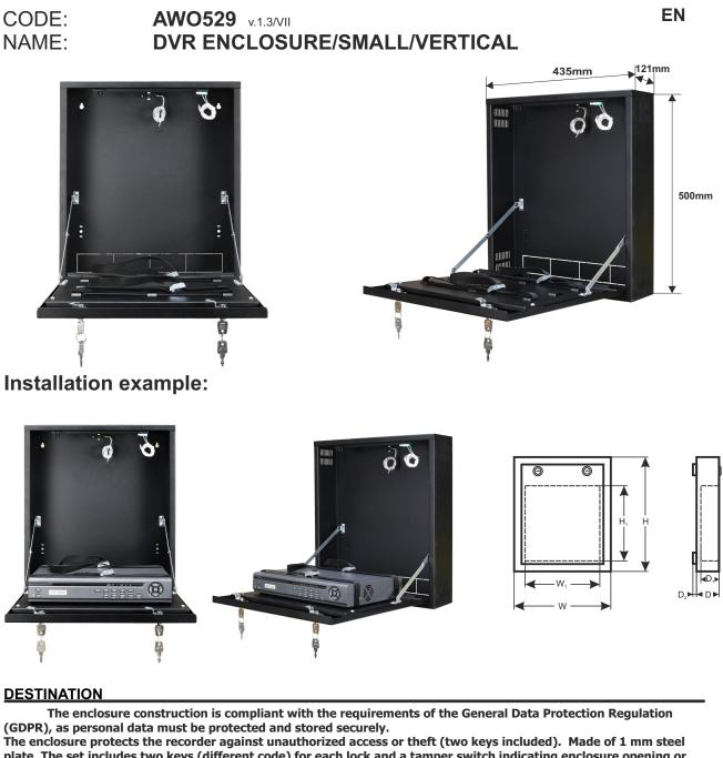
plate. The set includes two keys (different code) for each lock and a tamper switch indicating enclosure opening or unwanted removal of the enclosure from the wall.
